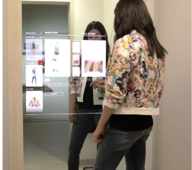
Consumer shows how this mirror display with RFID technology allows her to view various product lines.
